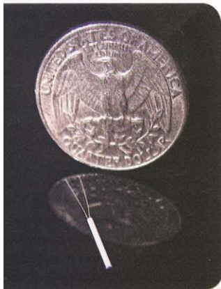
RTDs can be very small. This one uses ceramic encapsulation to protect the delicate platinum wires. If the mass is not too great, response time can still be kept short. Source: Heraeus Sensor Technology
